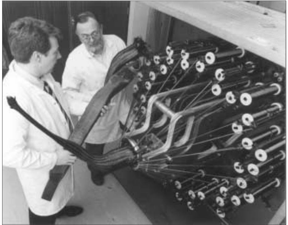
Triaxial braiding a test A-pillar preform for the Aston Martin Vanquish
